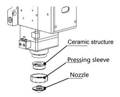
Fig 6.8 - Replace nozzle connector
