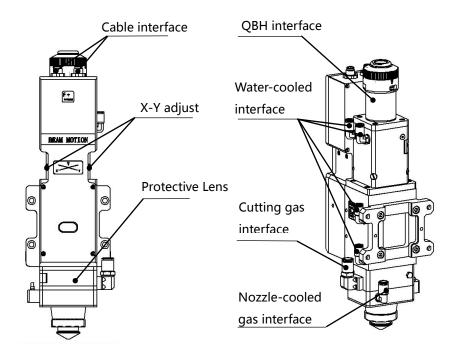
Fig 2.1 – Cutting head shape of BM111
