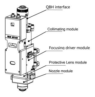
Fig 1 - laser head structure
