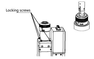
Fig 3.4 - Schematic diagram of fiber interface insert in QBH connector
