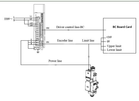
Figure 4.7 — Velocity loop FSCUT wiring diagram
