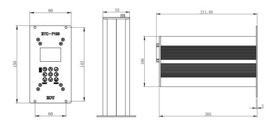
Fig 4.2 - ETC\_F100 Dimensions (Unit: mm)
