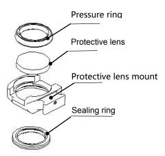
Fig 6.2 - Protective lens mount structure
