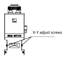
Fig 5.1 - QBH interface beam centering
