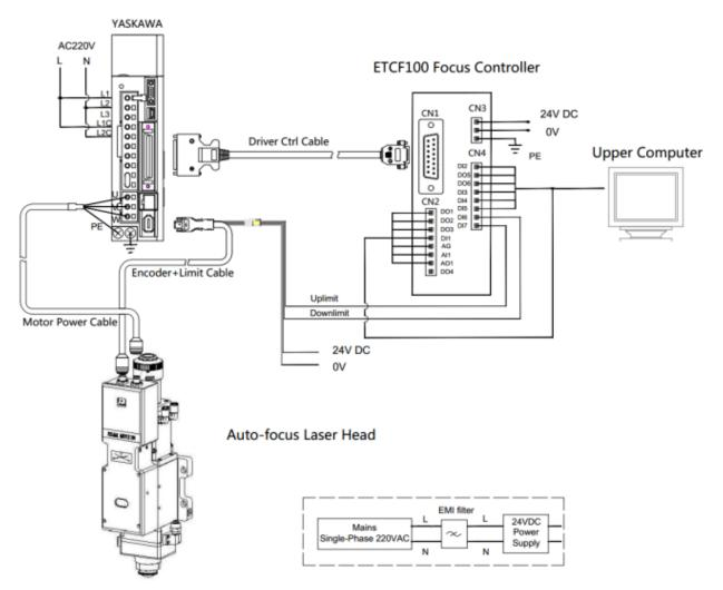
Note: The servo Ctrl cable, power cable, encoder cable + limit cable are standard cables. The CON2, CON3, CON4 interface cables should be prepared by the user.
