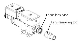
Fig 6.6 - Remove and install the focusing lens
