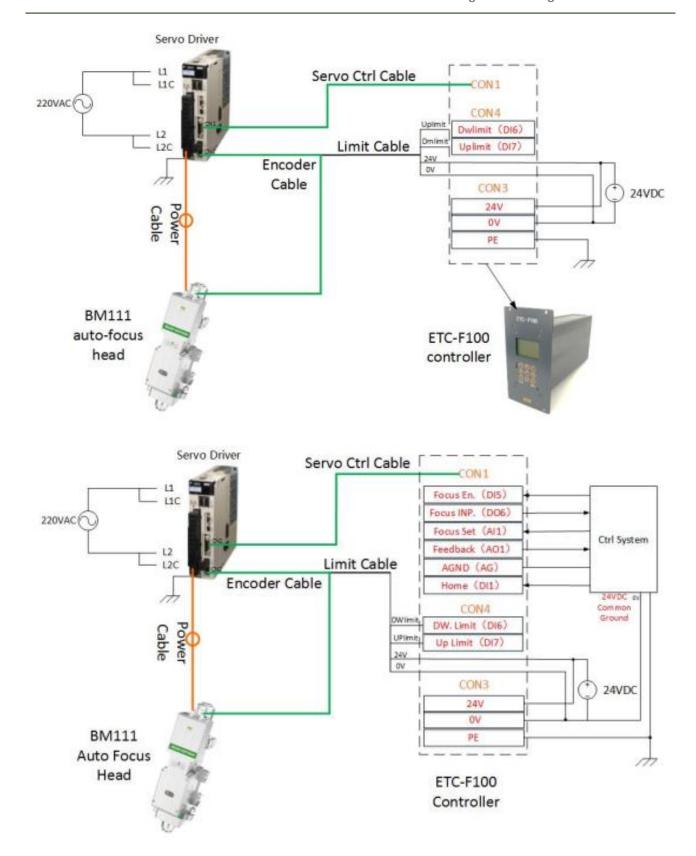
Fig 4.1 - BM111+ETC\_F100 Wiring
