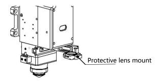
Fig 6.1 - Replace the protective lens
