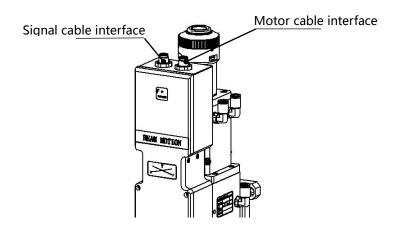
Fig 3.3 - cable interface of laser cutting head
