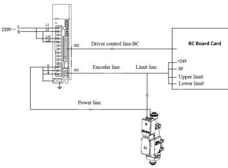
Figure 4.4 — Position loop FSCUT wiring diagram
