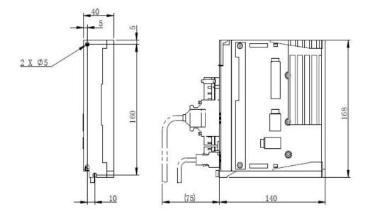
Figure 4.3 —Overall size of drive (unit: mm)
