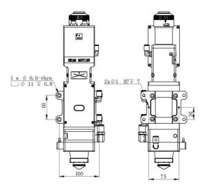
Fig 3.1 - mounting holes position
