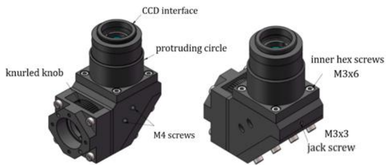
Fig. 2-4 CCD Adjustment
